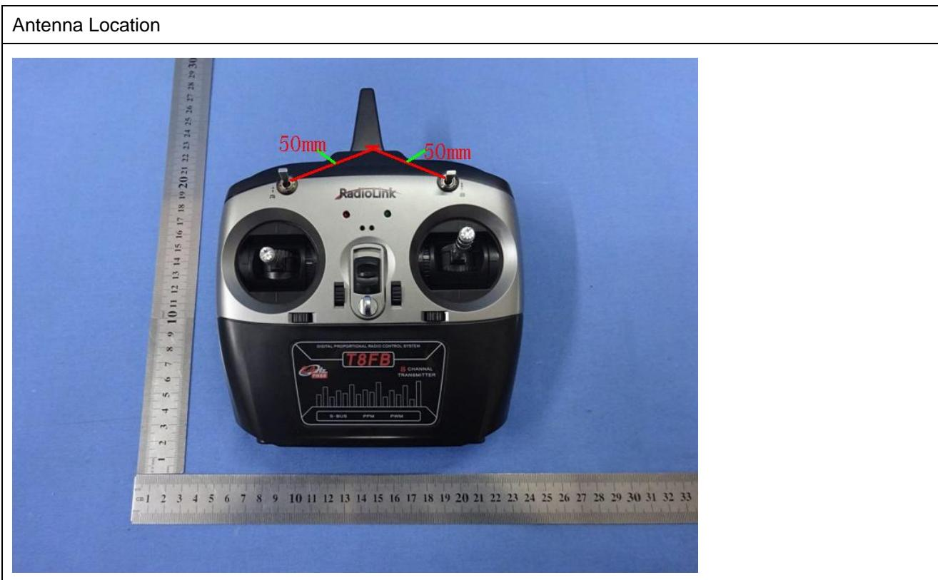
Refer to above photo, the minimum test separation is 50mm.
