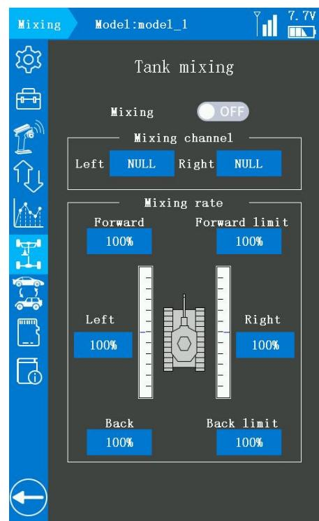
adjustment. The throttle channel and the steering channel operate in conjunction with each other. By operating the trigger to the high side, the car body advances as "Forward rate" while if operate the trigger to the brake side, the car body will backward as the "Back rate".
