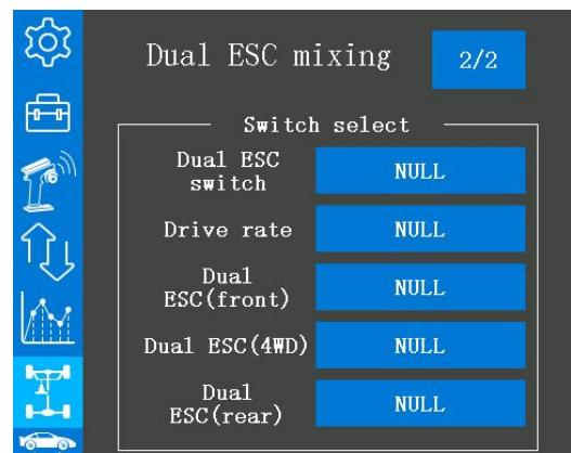
As this function drives 2 separate motors simultaneously, a mutual load will be applied. Use this function carefully so that the motors are not damaged.
