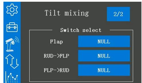
**FLP->RUD:** DT1/DT2/DT3/DT4/DL1 can be selected to adjust the mixing amount from flap to rudder.
