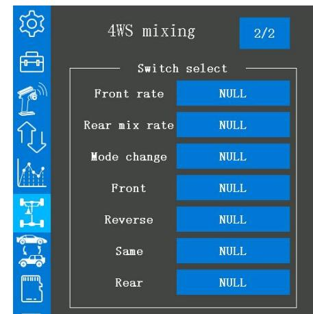
DT1/DT2/DT3/DT4/DL1 can be set to switch from front-drive only, rear-drive only, and both front and rear drive (4WD), or select one of the buttons PS1/PS2/PS3/PS4/PS5/Steering/ Trigger to trigger one of the Dual ESC types.
