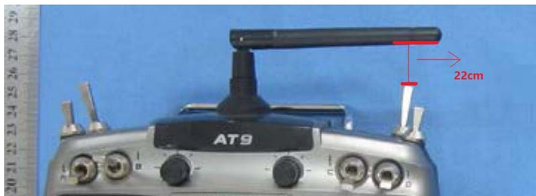
Shortest distance between antenna and switch is 22cm
