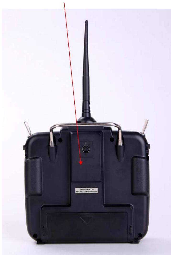
The label shown shall be permanently affixed at a conspicuous location on the device and be readily visible to the user at the time of purchase (Labeling requirements per 2.925)
