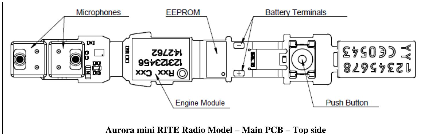
The most important part of the radio model is the Engine Module mounted on the main flex PCB, which connects it to both the EEPROM memory and all external connections: On the top side these are the microphones, the battery terminals and the push button.
