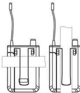
Clip the transmitter to a belt through the transmitter clip as show.
