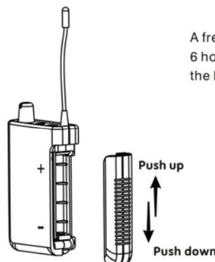
A fresh alkaline battery lasts up to 6 hours. When the LED flashed RED, the battery should be replaced.
