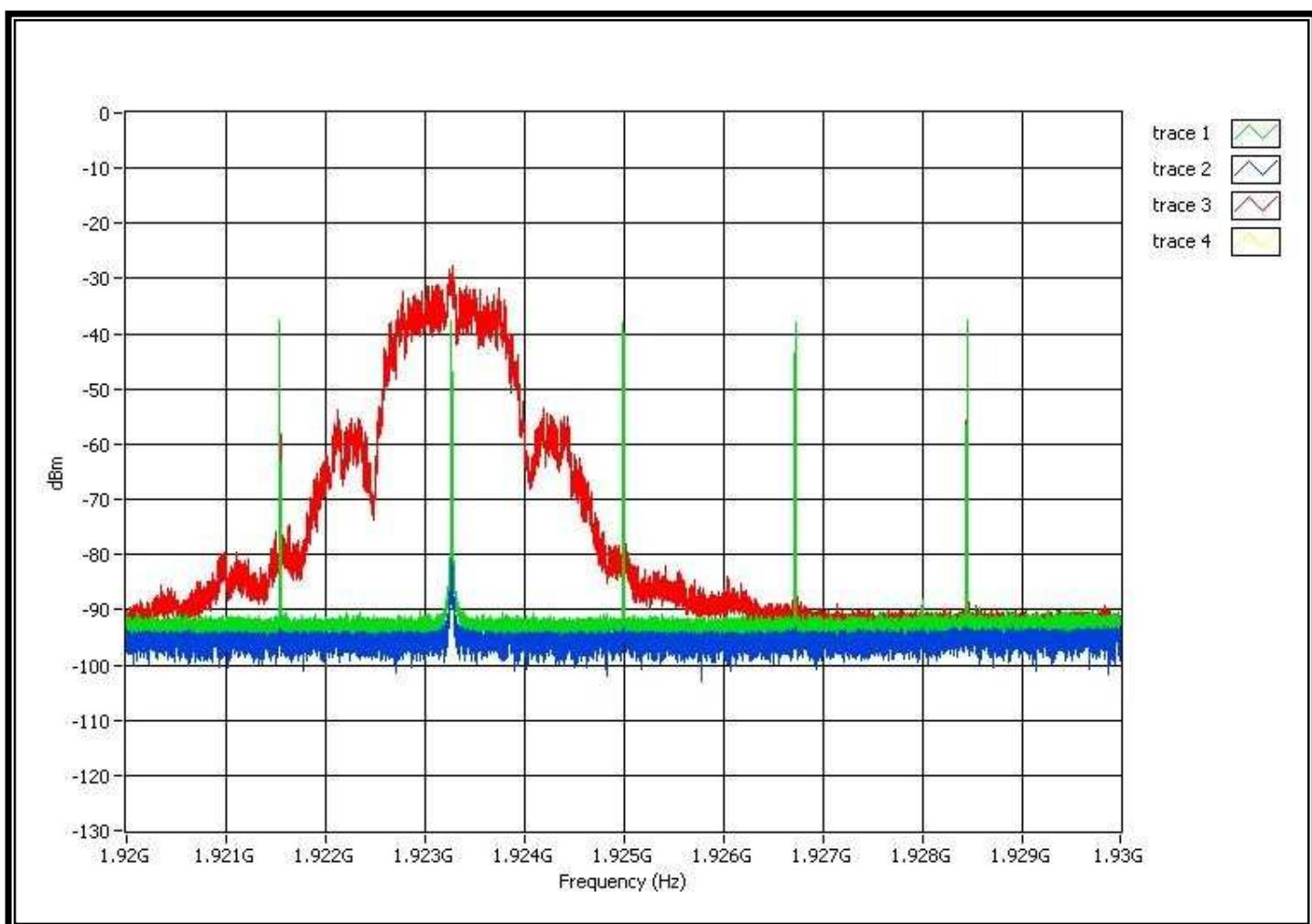
Note1: Trace1 (green) is the interference on all 5 carriers. The level is  $T_u+U_m+10$ dB.
