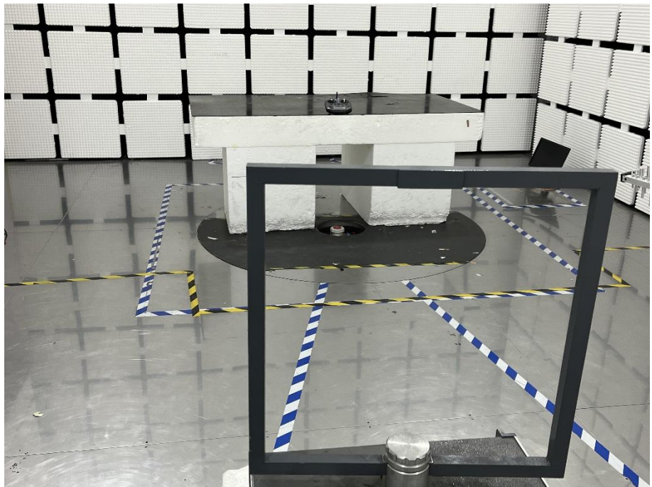
Radiation Emission Test Setup (Below 30MHz)
