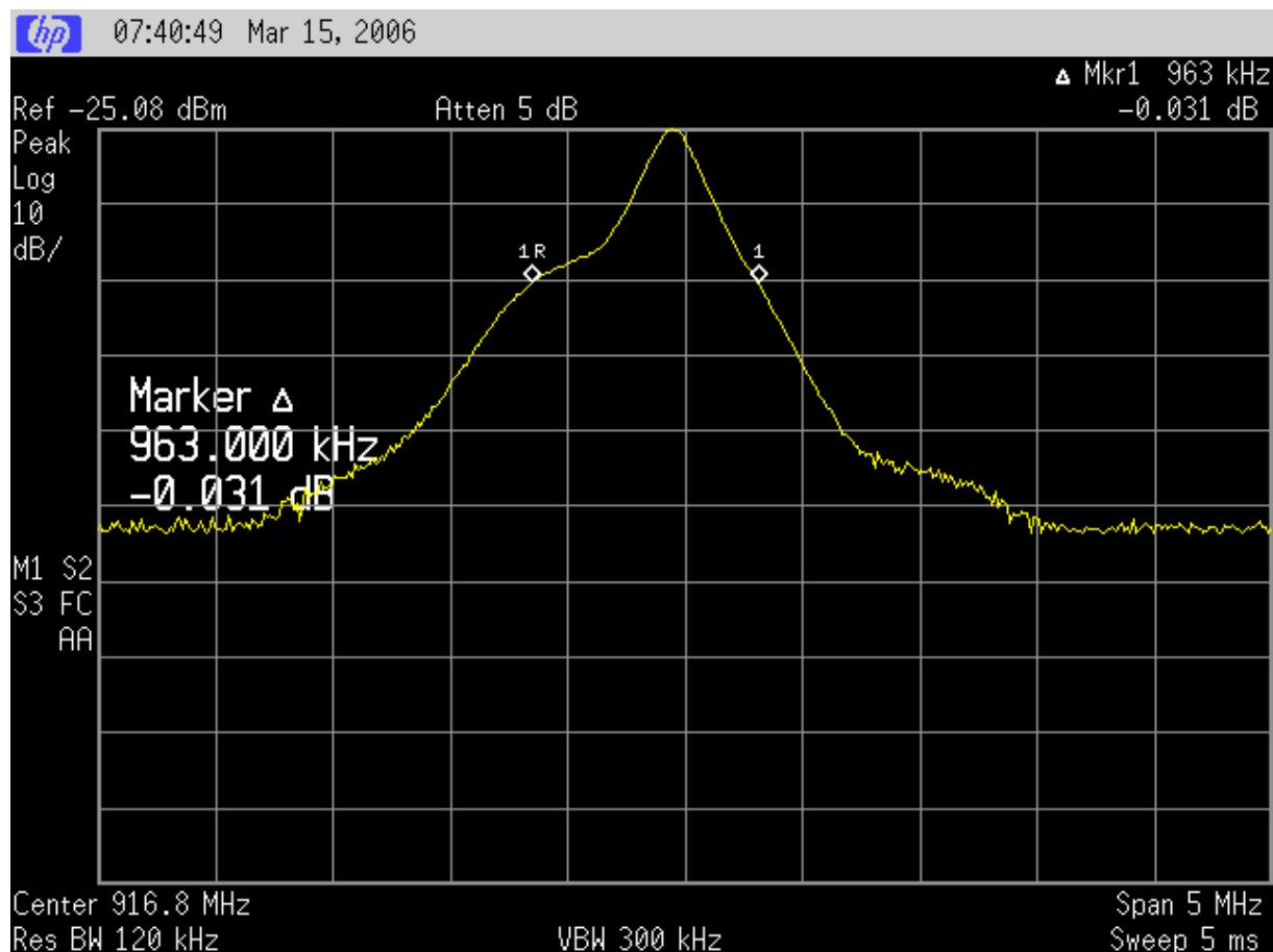
The spectrum plot shows that the 20 dB bandwidth is completely contained within the allocated band of 902 – 927 MHz.
