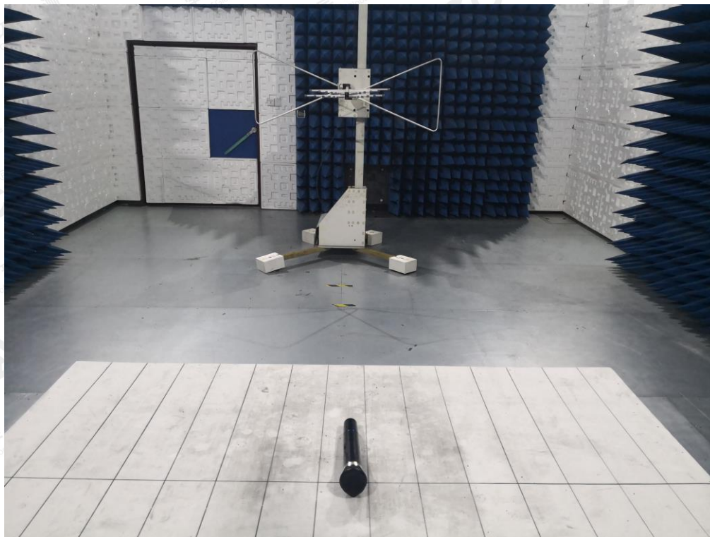
RADIATED EMISSION TEST SETUP ABOVE 1GHZ
