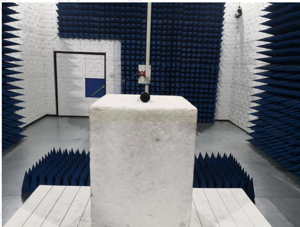
RADIATED EMISSION TEST SETUP ABOVE 1GHZ
