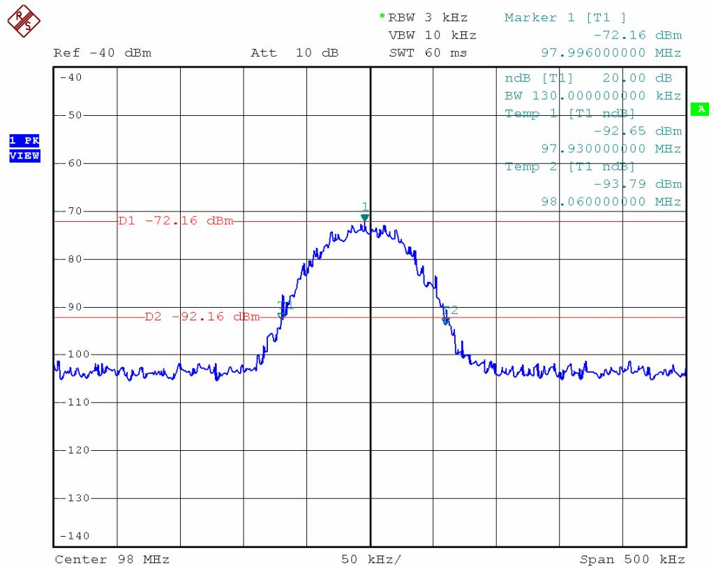
20dB bandwidth of the emission is 130.0 kHz
