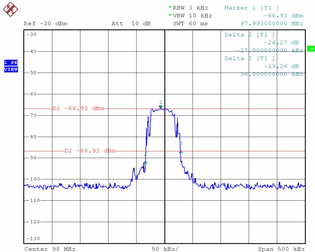
20dB bandwidth of the emission is 63.0 kHz
