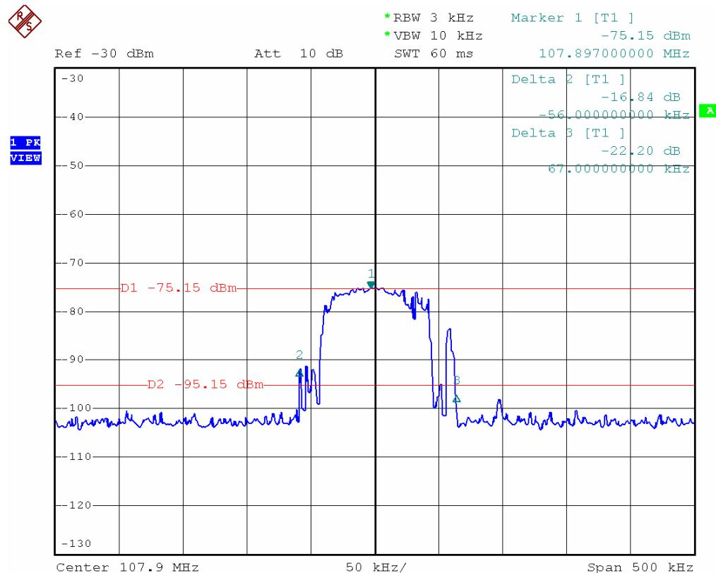
20dB bandwidth of the emission is 123.0 kHz
