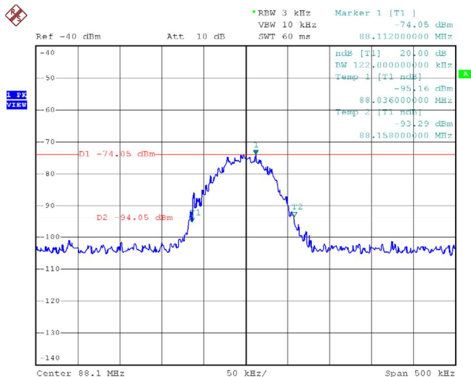
20dB bandwidth of the emission is 122.0 kHz.
