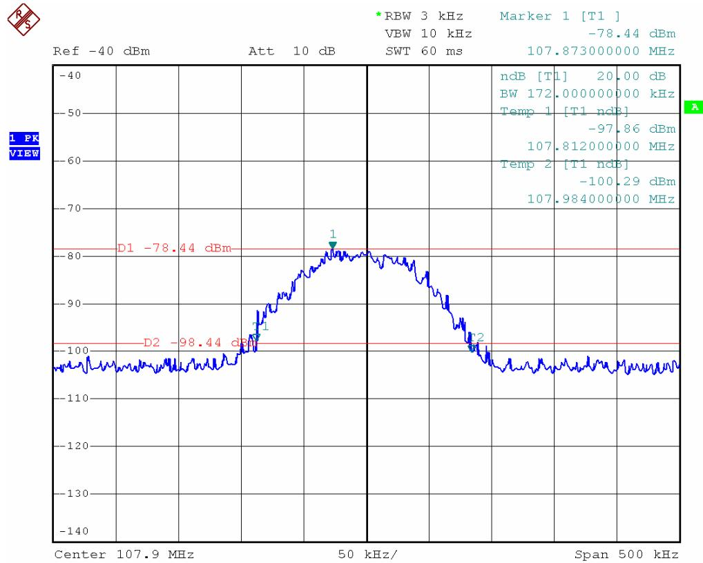
20dB bandwidth of the emission is 172.0 kHz
