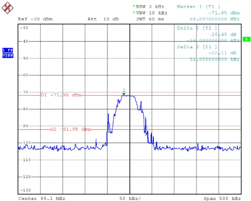
20dB bandwidth of the emission is 87.0 kHz.
