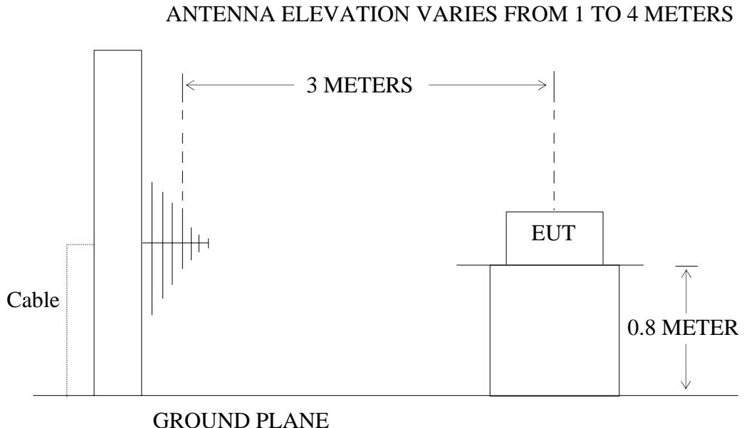
(EUT: FM Transmitter For iPod)
