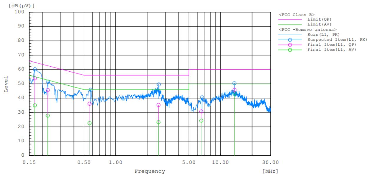
**AC Line Conducted Emission (N) : RF output terminated with dummy load**
