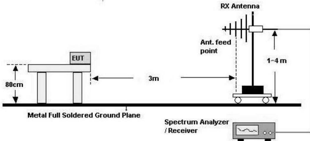
**Test Procedure of Radiated spurious emissions (Below 1GHz)**
