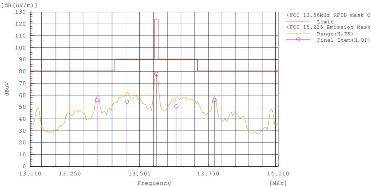
Radiated E-Field Emission (Antenna Position 90°) : 13.110 – 14.010 MHz
