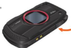
6. Make sure the port cover is completely closed.
