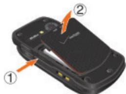
3. Remove the battery by pulling the tab vertically up.
