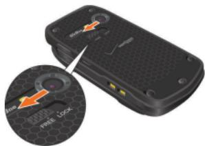
2. Insert your finger in the groove ① and pull up on the battery cover in the direction of the arrow ②.
