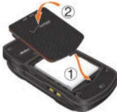
**5.** Press down firmly on the sides of the battery cover at each arrow point, as shown to the right.
