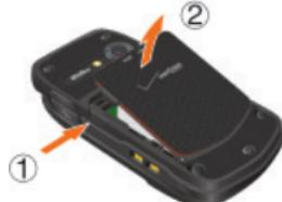
**3.** Slide the battery into the slot by aligning the contacts and tabs ① and press down ② until you hear the "click".
