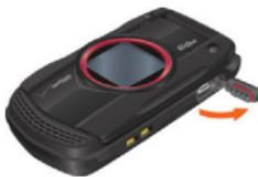
2. Connect the small connector of the USB Cable (included in box) into the Charging/Data Port.
