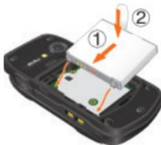
**4.** Insert the battery cover tabs into the slots ① and press the battery cover in the direction of the arrow ②.
