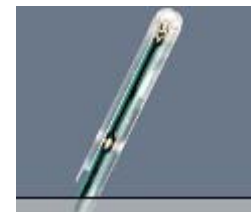
Figure 5-2 H-Field Free-space Probe
