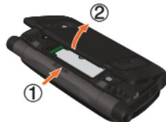
**4.** Insert the two tabs on the left side of the battery into the cellphone (in the direction of the arrow ① in the figure to the right) and insert the battery into the cellphone (in the direction of the arrow ② in the figure to the right).
