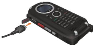
3. When the cellphone is completely charged, unplug the Wall Charger connector and push the center of the port cover into the Charging/Data Port.
