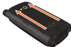
**7.** Slide the Battery Cover Lock to the LOCK position in the direction of the arrow in the figure to the right.
