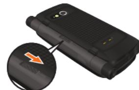
2. Insert your nails of the thumb in the recesses of the battery cover indicated with arrows in the figure to the right, and slightly move its both ends up.
