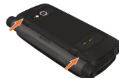
**3.** Insert your fingertip into the recess ①, and then pull the battery cover up to the direction ② as indicated in the figure to the right.
