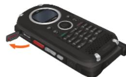
2. Plug the Wall Charger power plug into an electrical outlet and the Wall Charger connector to the Charging/Data Port.
