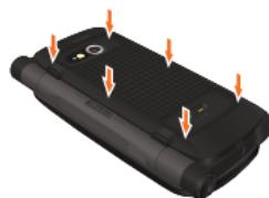
**6.** Slide your finger over both sides of the battery cover in the direction of the arrow and check that the battery cover is firmly in place.
