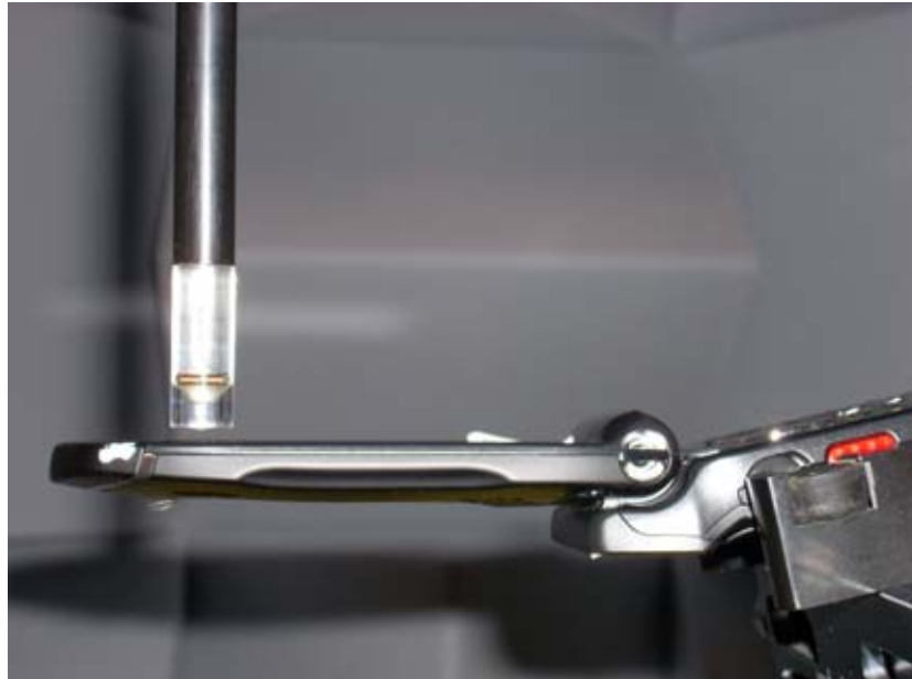
Figure 13-1 Test Setup for Wireless Device
