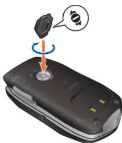
2. Insert the tip of the corner of the Device Lock Tool marked with the battery lock icon
