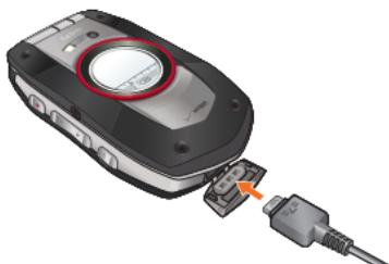
You can also charge the battery by directly connecting the AC Charger to the Accessory Connector Port located at the bottom of the handset.
