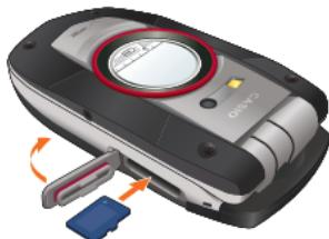
2. Carefully press the memory card into the slot until it locks into place.
