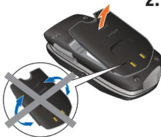
Do not twist the battery as shown in the illustration. Doing so can damage the phone and the battery.
