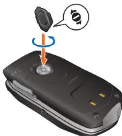
1. Insert the tip of the corner of the Device Lock Tool marked with the battery lock icon
