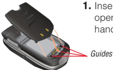
1. Insert the battery into the opening on the back of the handset using the guides.
