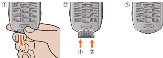
**Warning!** Failure to completely reseal the Accessory Connector Port after charging may result in damage if the phone is exposed to water.
