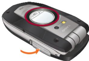
**Warning!** Failure to fully close the memory card slot cover after installing or removing a memory card can allow water to leak inside and create the risk of malfunction.
