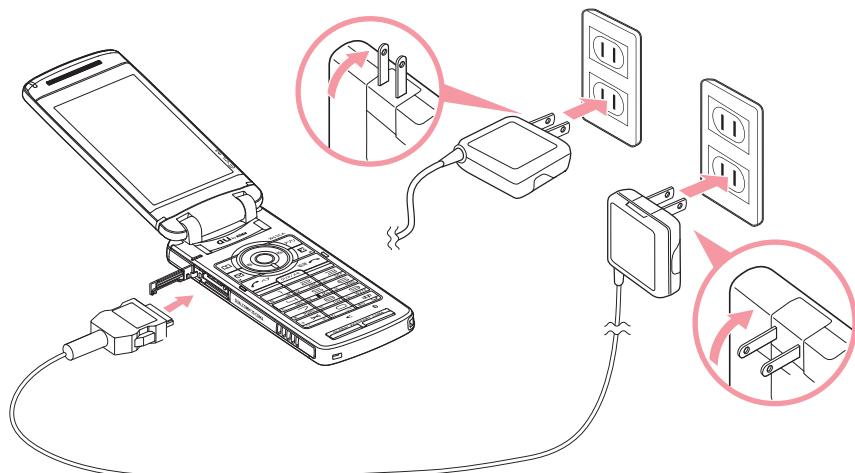
Fully open the external connection jack cover, check the shape of connectors and insert it horizontally.
