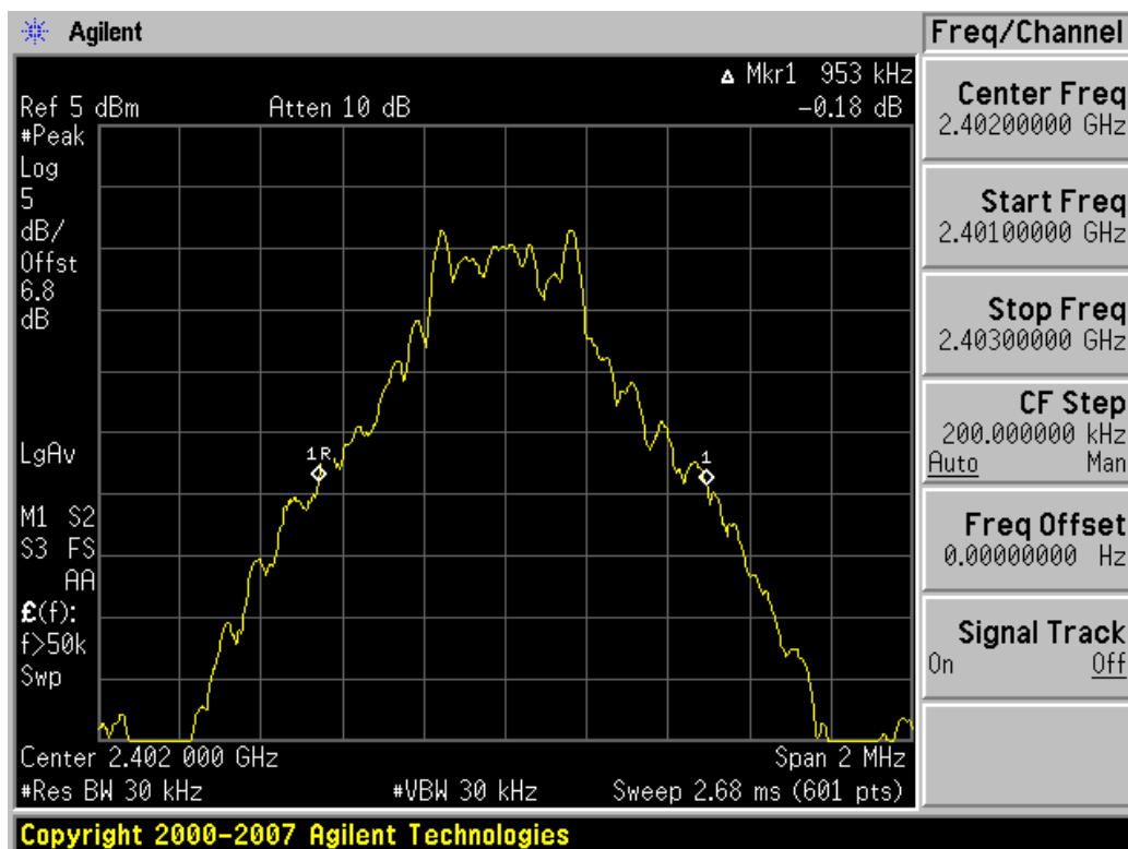
Plot 6-1. 20dB Bandwidth Plot (Bluetooth, 1Mbps – Ch. 0)
