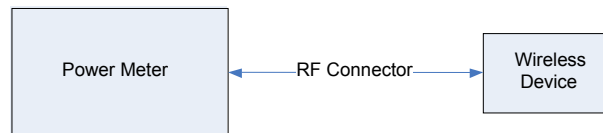
Figure 12-1 Power Measurement Setup
