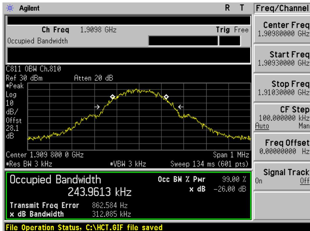
■ GSM1900 EDGE (512 CH.) Occupied Bandwidth
