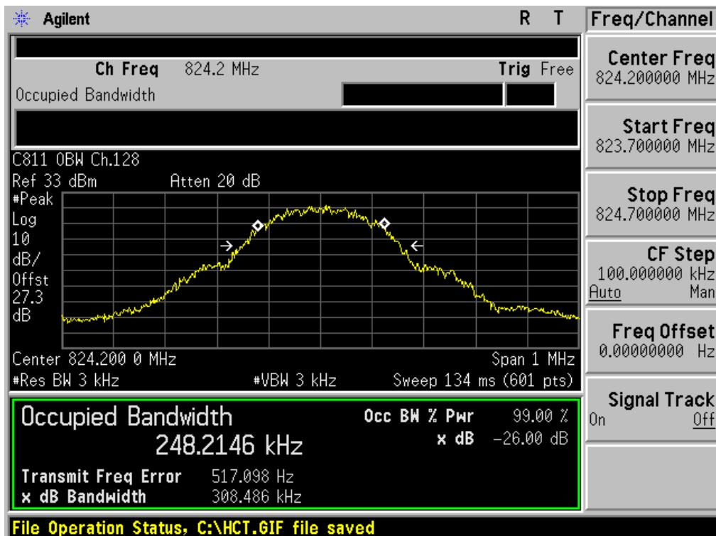
■ GSM850 MODE (190 CH.) Occupied Bandwidth
