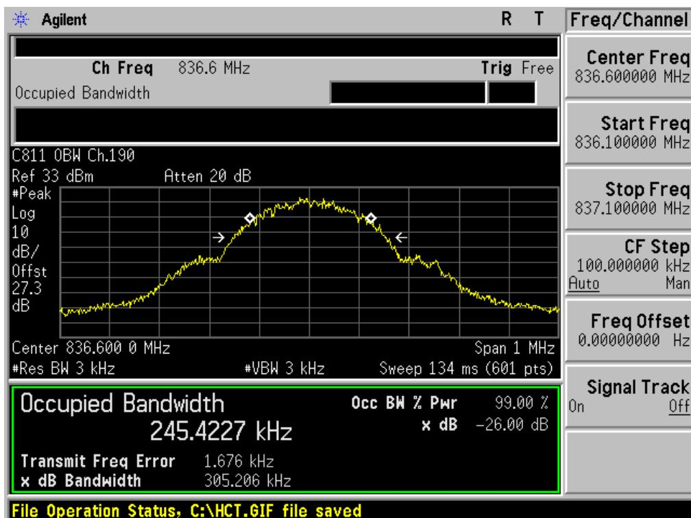
■ GSM850 MODE (251 CH.) Occupied Bandwidth
