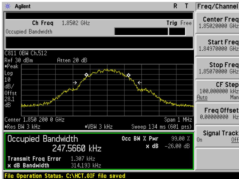
■ GSM1900 MODE (661 CH.) Occupied Bandwidth
