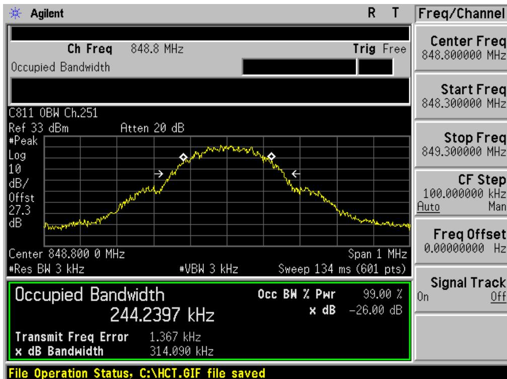
■ GSM850 EDGE (128 CH.) Occupied Bandwidth
