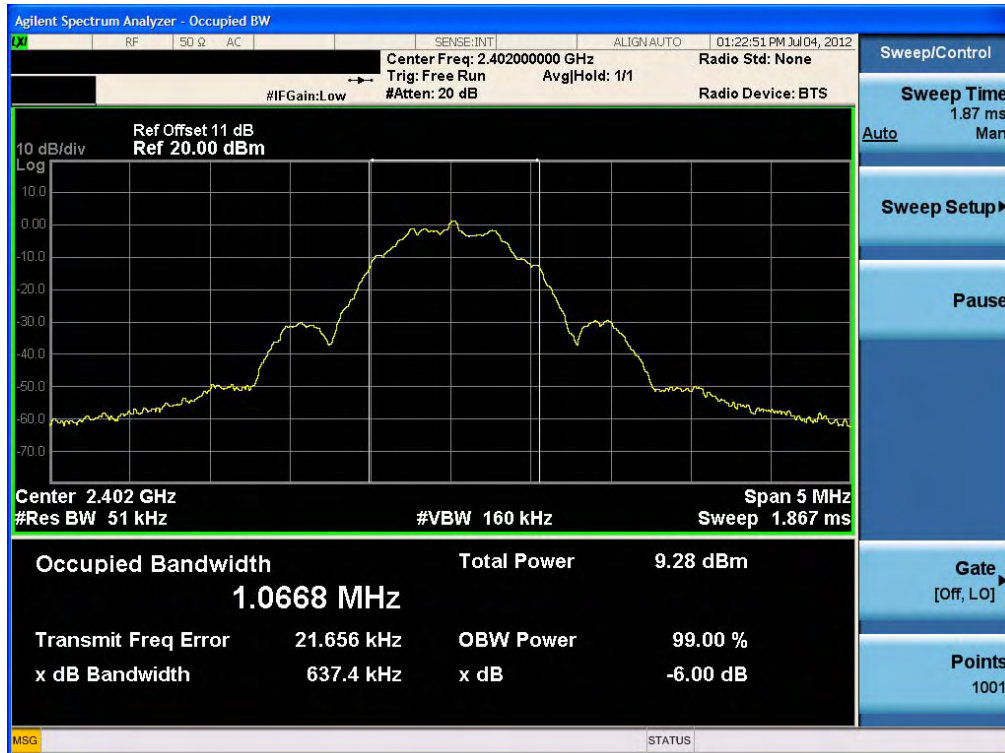
6dB Bandwidth plot (Low-CH 0)
