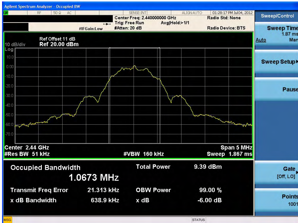
6dB Bandwidth plot (Mid-CH 19)
