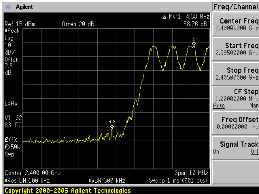
Test Plots with hopping (GFSK)
