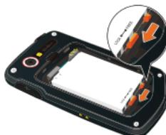
To remove the battery, pull up the tab.
