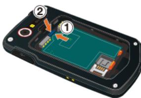
**3.** Remove the microSD card from the microSD card slot as shown in the right figure.
