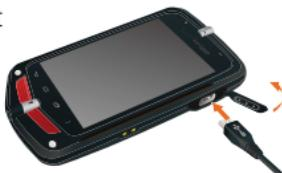
2. Connect the opposite end of the USB Cable to the USB port on the Wall Charger (included in box).
