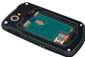
**4.** Install the battery and replace the battery cover making sure to slide the Battery Cover Lock to the LOCK position.
