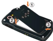
3. To install the battery, slide the battery into the slot by aligning the contacts and tabs ① and press down ② until it fits into place. Fold down the battery tab toward the battery.
