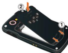
5. Press down firmly on all sides of the battery cover at each arrow point, as shown in the right figure.
