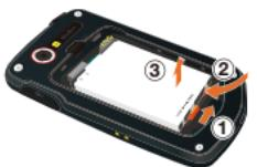
4. Insert the battery cover tabs into the slots ① and press the battery cover in the direction of the arrow ②.
