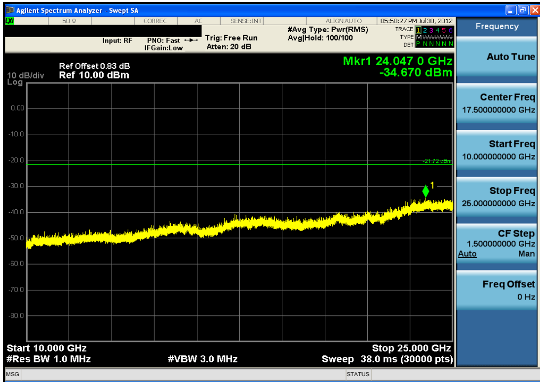
Plot 6-19. Conducted Spurious Plot (Bluetooth, 1Mbps – Ch. 0)
