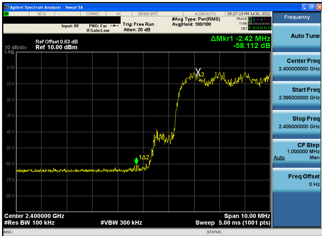
Plot 6-12. Band Edge Plot (Bluetooth with Hopping Enabled, 1Mbps)
