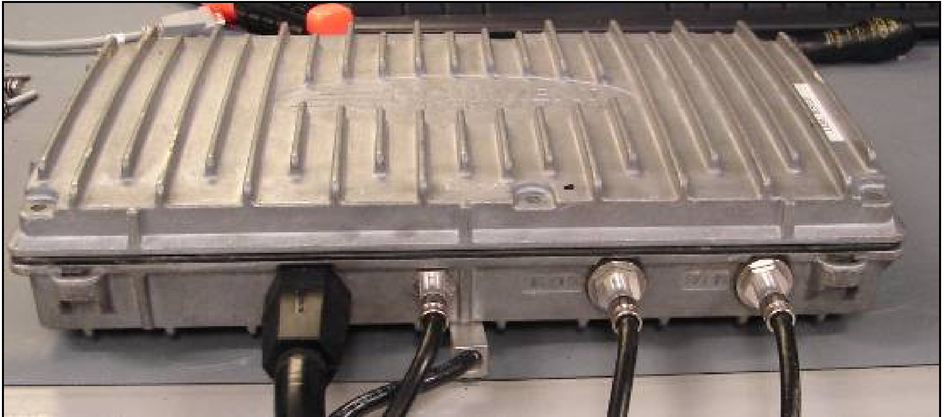
Photograph EP-1: External Photo of CT Bridge® URD 5010mvx – View of Front Side and connectors
