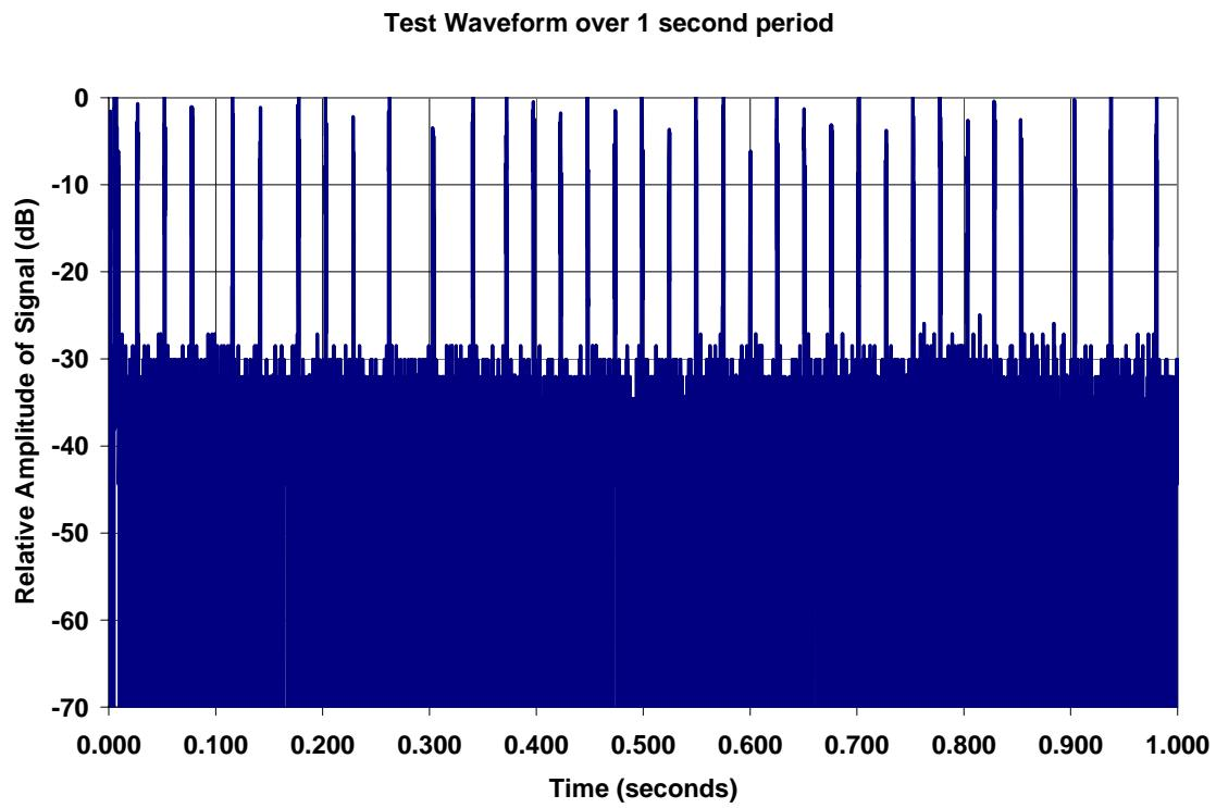
The repeated bursts ensure that the quasi-peak filter decay constant is not allowed to fully discharge, thereby ensuring that the measurement will register the maximum possible emissions as called out in Appendix C.
