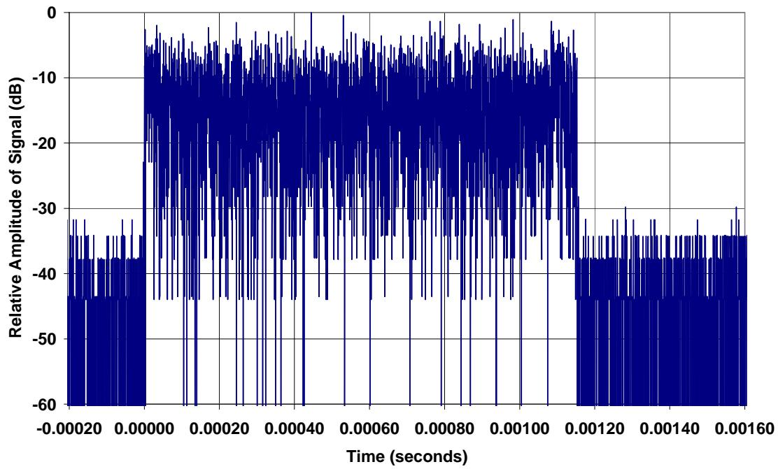
Note that the burst is longer than 1 ms, ensuring that the signal remains continuously on during the rise time of quasi-peak detection filter.
