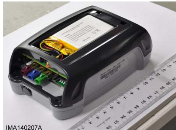
Internal Battery Location
