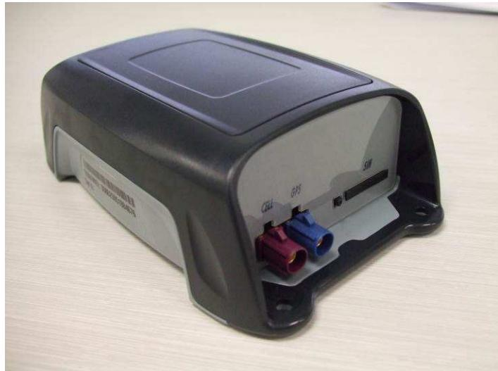
The endplate of 301-IX is different to cover the lack of Wi-Fi connectivity, note no Green FAKRA connector.
