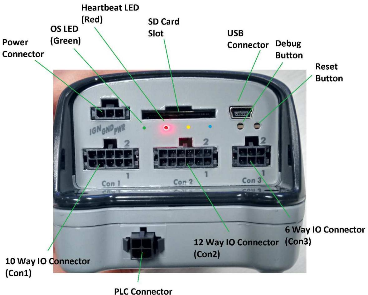
**NOTE:** The Vector 301 XWP is shown. The Vector 301 IW looks identical to the picture shown here, without the larger grey base holding the PLC Interface.
