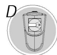
Select FM frequency by rotating the frequency knob at the side of the transmitter.
