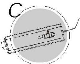
Play Mp3 or CD player and switch on the Power switch of the FM transmitter on the rear.
