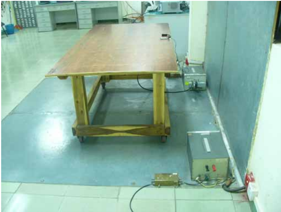
Conducted Emission Setup Photo – Side View
