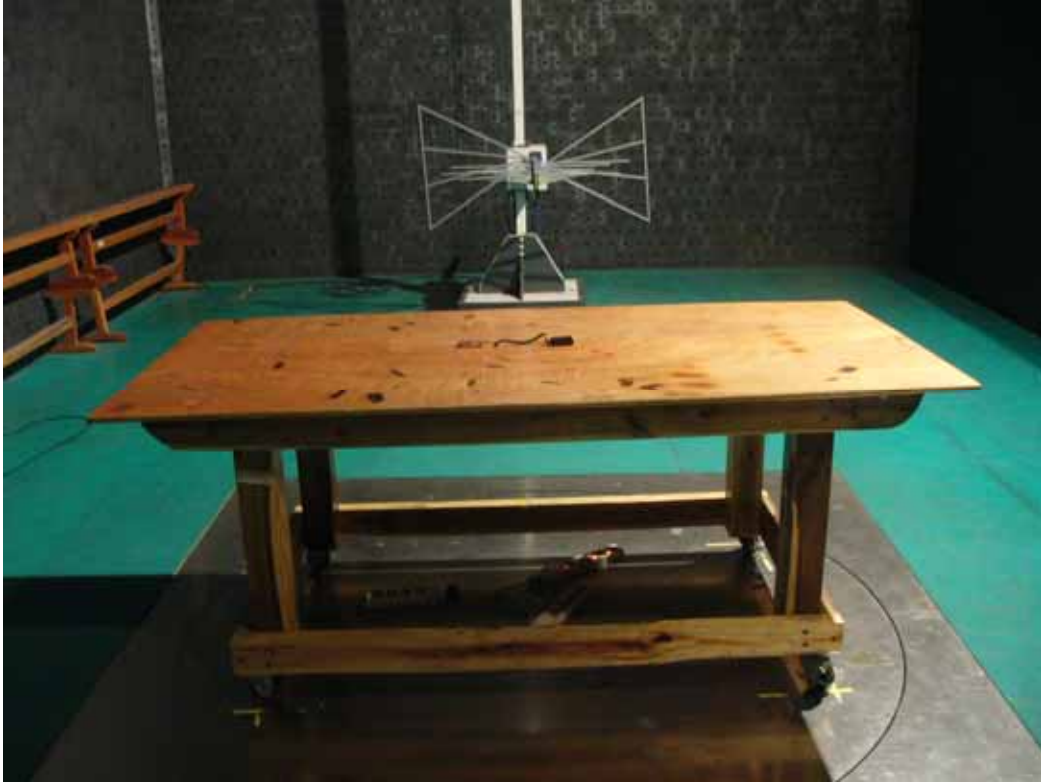
Radiated Emission Setup Photo
