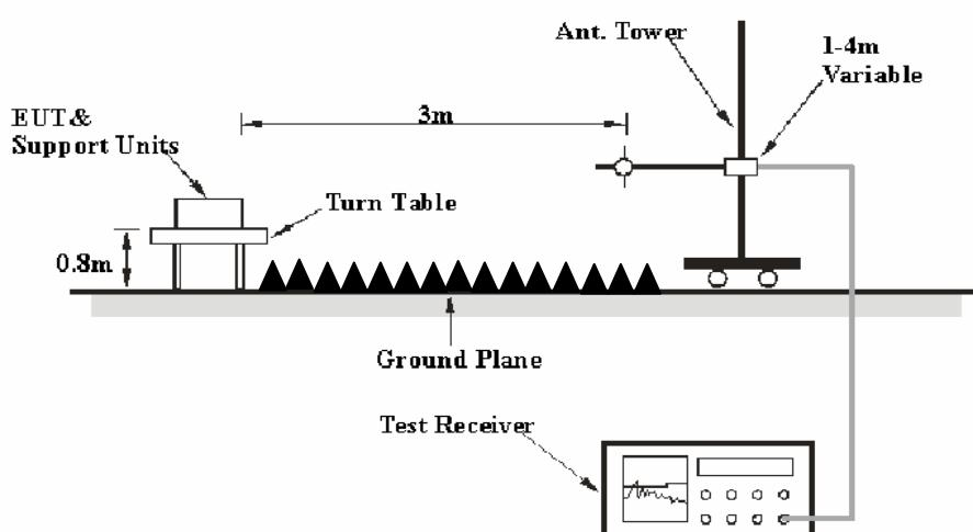
The radiated emission tests were performed in the 3 meters test site, using the setup accordance with the ANSI C63.4 - 2009. The specification used was the FCC 15 § 15.209, 15.205 and 15.231.
