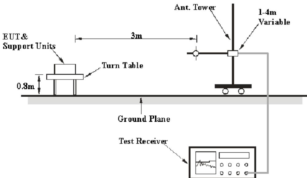
The radiated emission tests were performed in the 3 meters chamber B test site, using the setup accordance with the ANSI C63.4 - 2003. The specification used was the FCC 15 §15.209 and 15.231.
