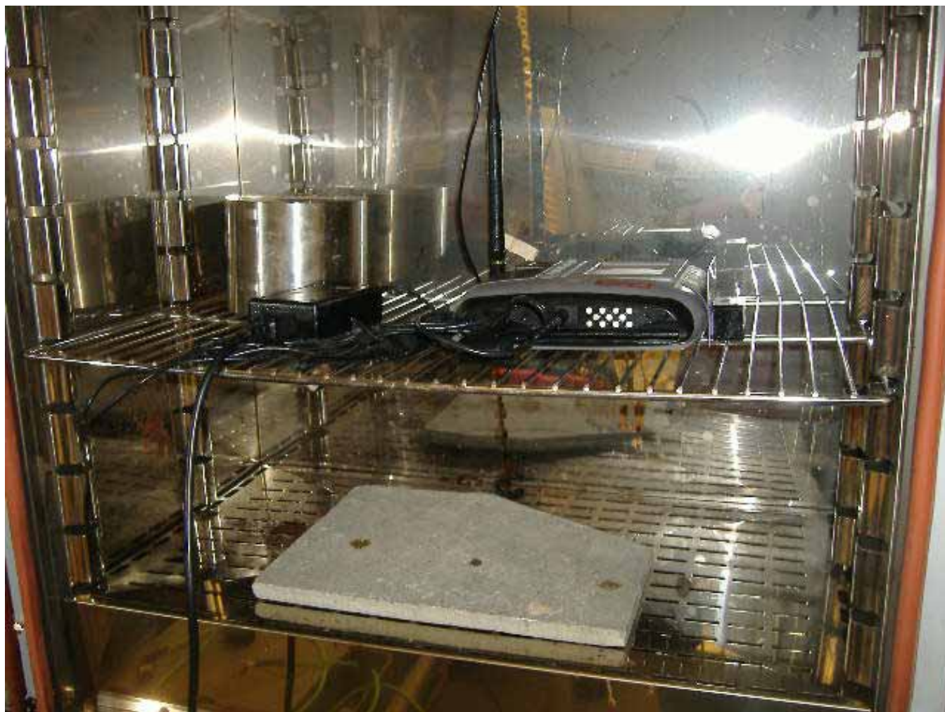
Figure 9 +50°C Temperature Test Setup
