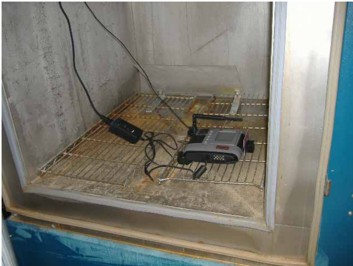
Figure 8 —20°C Temperature Test Setup
