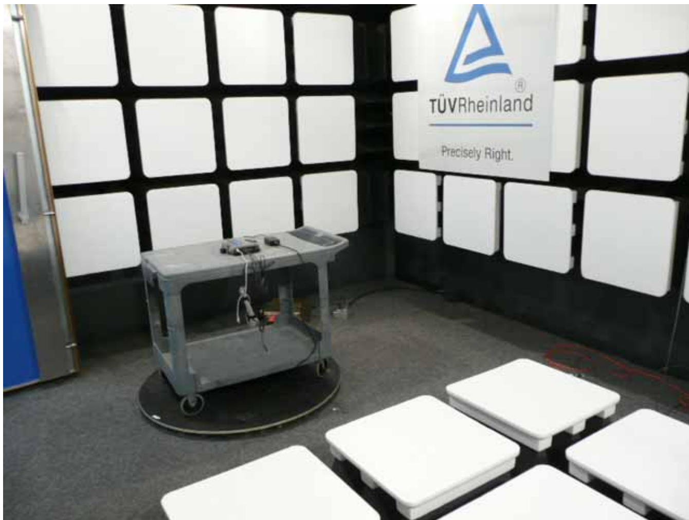
Figure 4 – Prescan Radiated Field Strength Emissions Test Setup (Semi-Anechoic Chamber)
