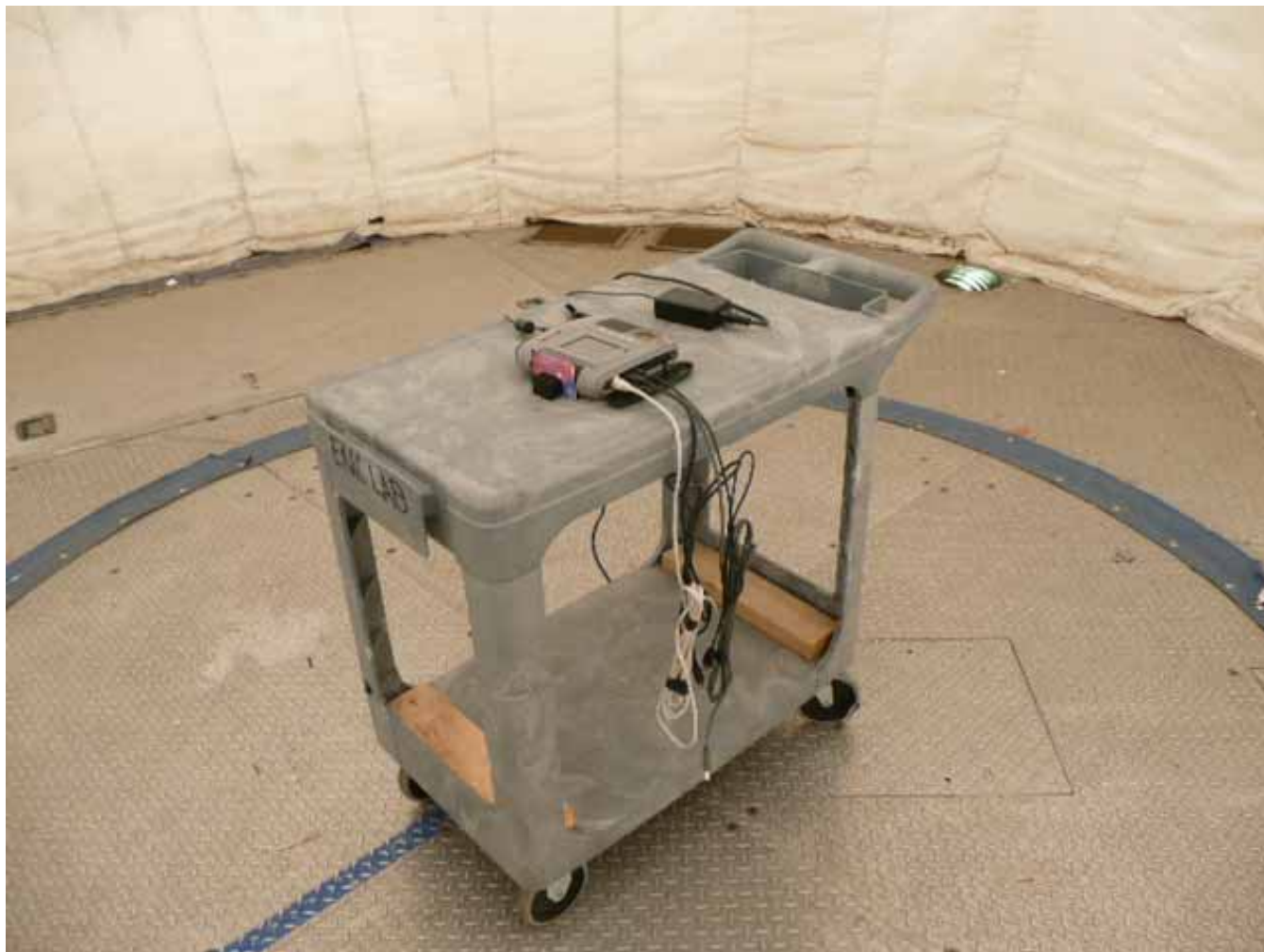
Figure 3 - Radiated Field Strength Emissions Test Setup O.A.T.S.
