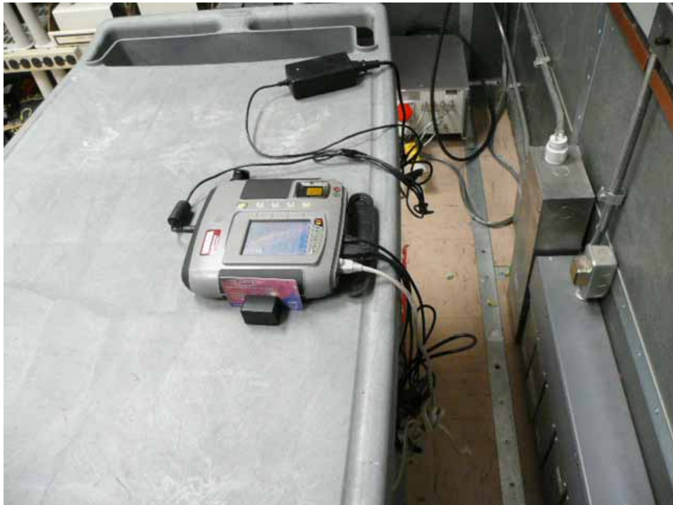
Figure 7 –Conducted Emissions Test Setup (back)
