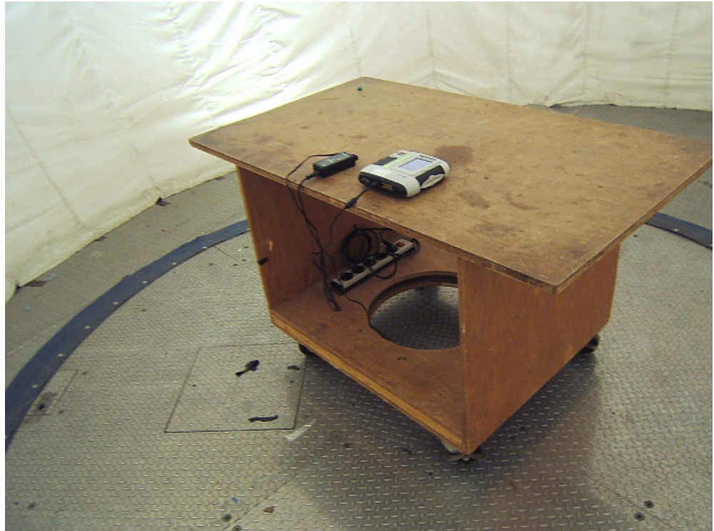
Setup for Radiated emissions and Field Strength emissions on 10 meter OATS – Final test
