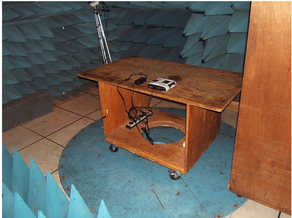
Setup for Radiated emissions Prescan in Anechoic Chamber
