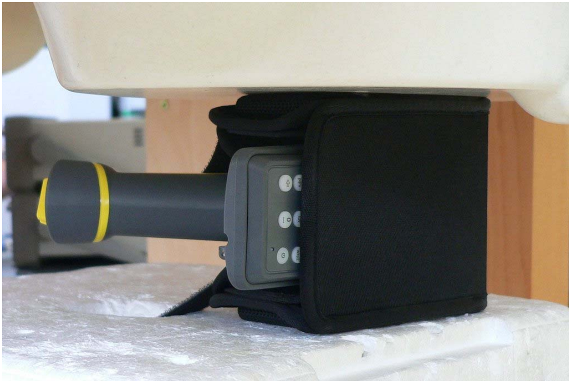
Fig. 16: Body worn configuration, position 1 with holster, left edge of display in direct contact against the flat phantom.
