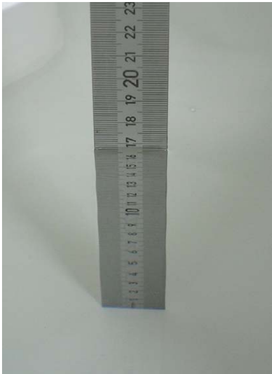
Fig. 18: Liquid depth for IEEE 802.11 b/g Body measurements
