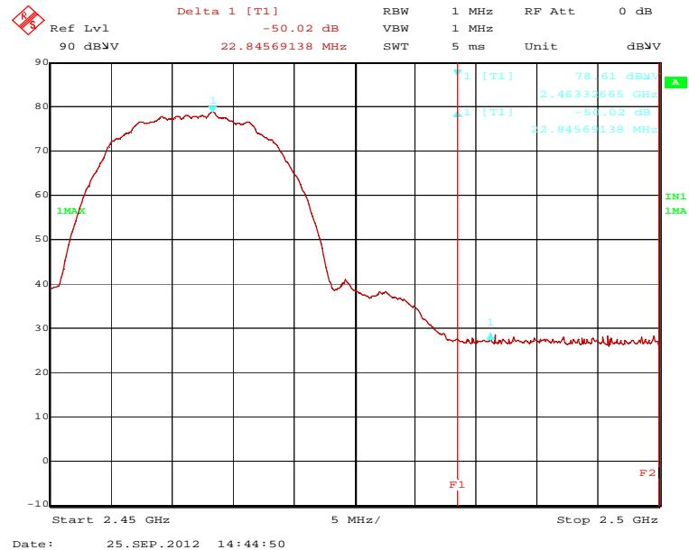
123441\_7.wmf: Radiated band-edge compliance, upper band edge (operation mode 6):
