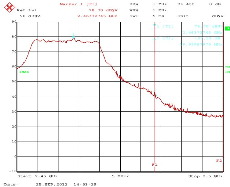
The plots on the pages before are showing the radiated band-edge compliance for the lower and upper band-edge. The frequency line 1 (F1) shows the upper and the frequency line 2 (F2) shows the lower edge of the assigned frequency band.
