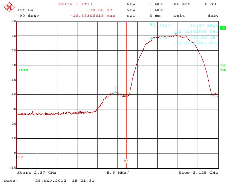
123441\_8.wmf: Radiated band-edge compliance, lower band edge (operation mode 4):
