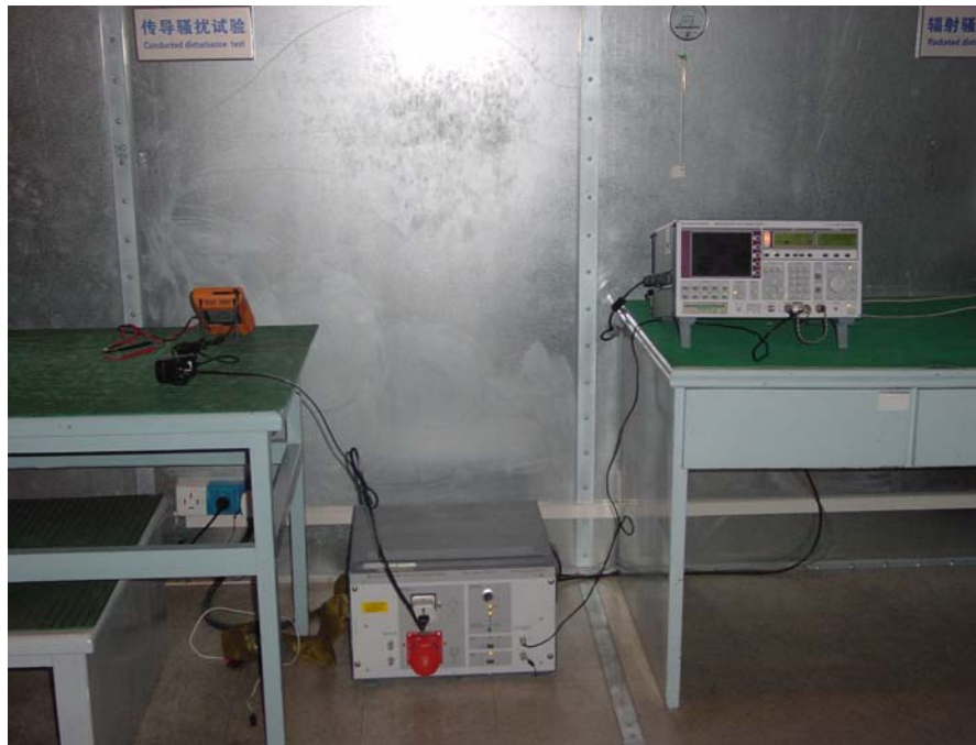
Conducted Emission Test Set-up Front View
