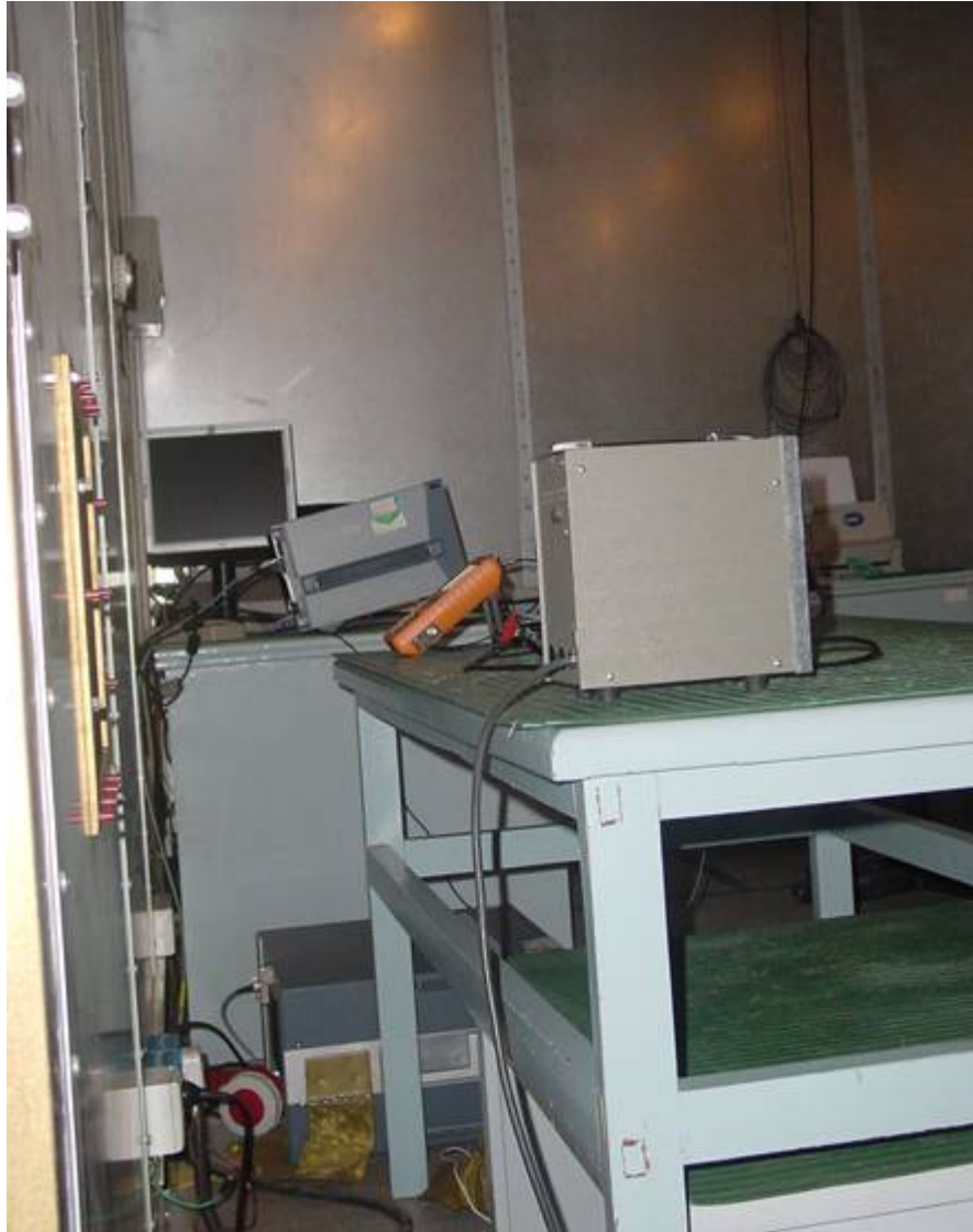
Conducted Emission Test Set-up Side View
