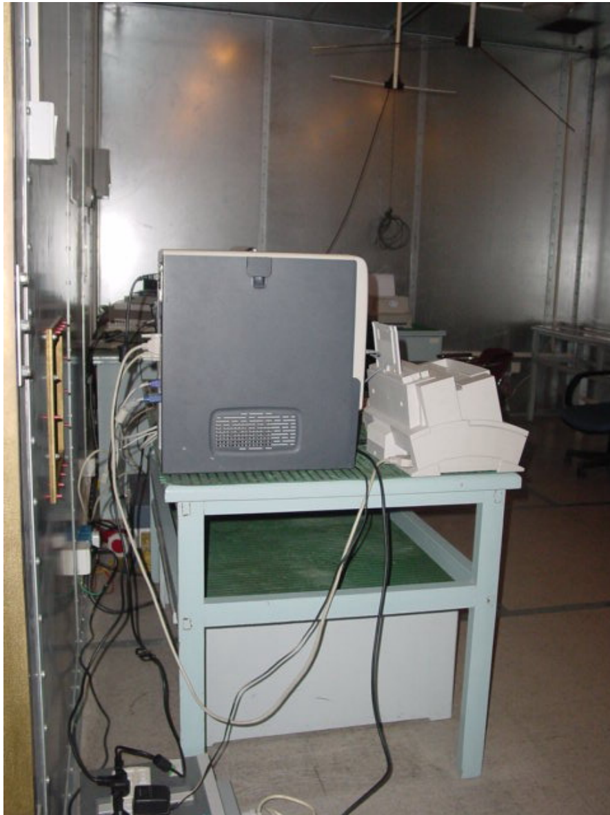
Conducted Emission Test Set-up Side View
