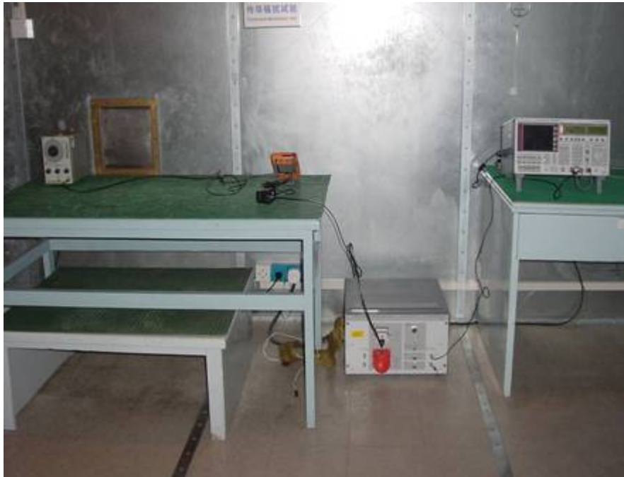
Conducted Emission Test Set-up Front View
