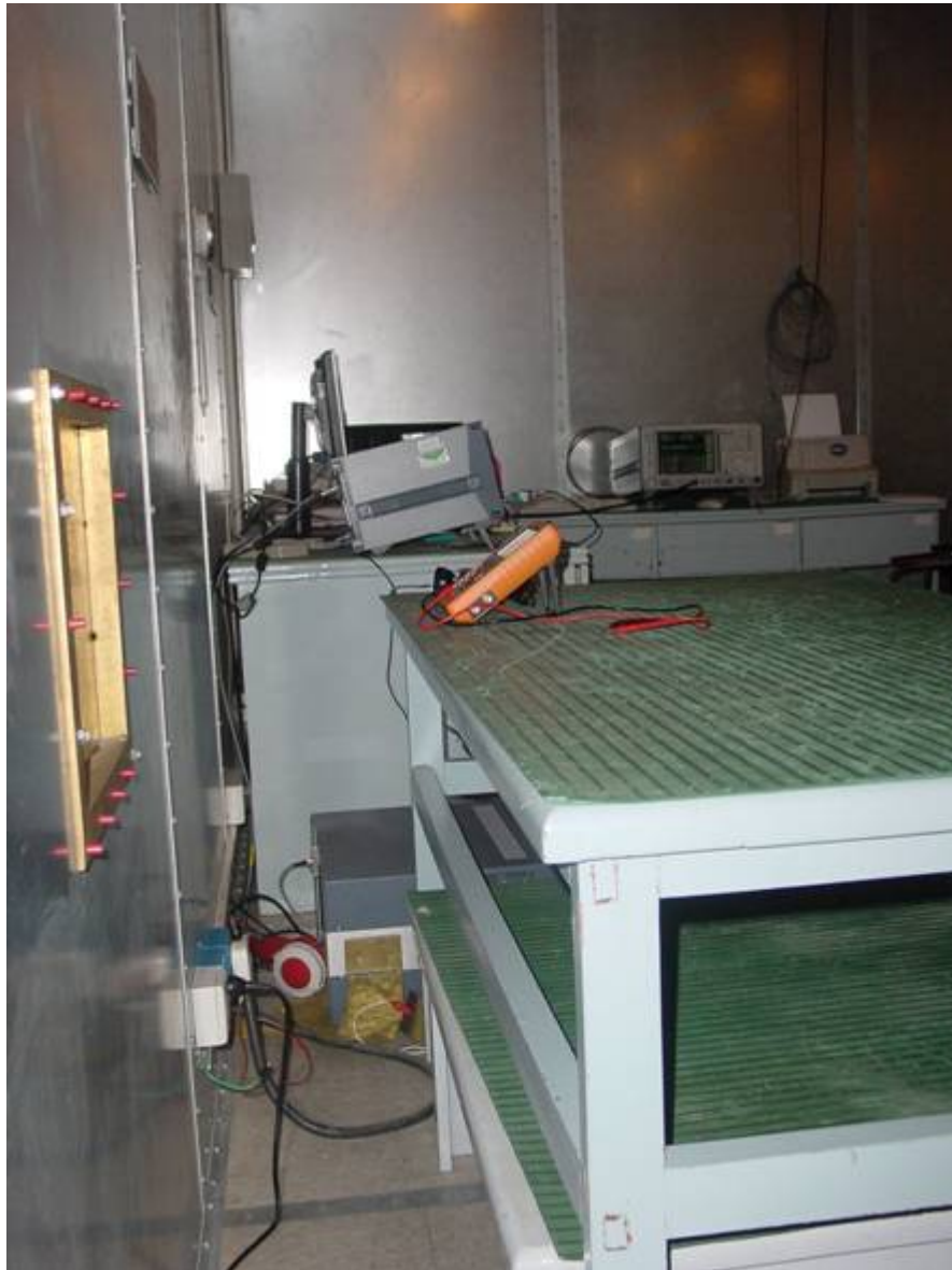
Conducted Emission Test Set-up Side View
