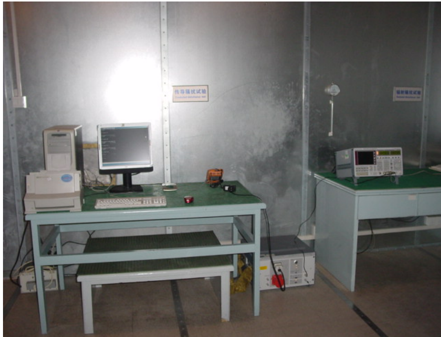
Conducted Emission Test Set-up Front View
