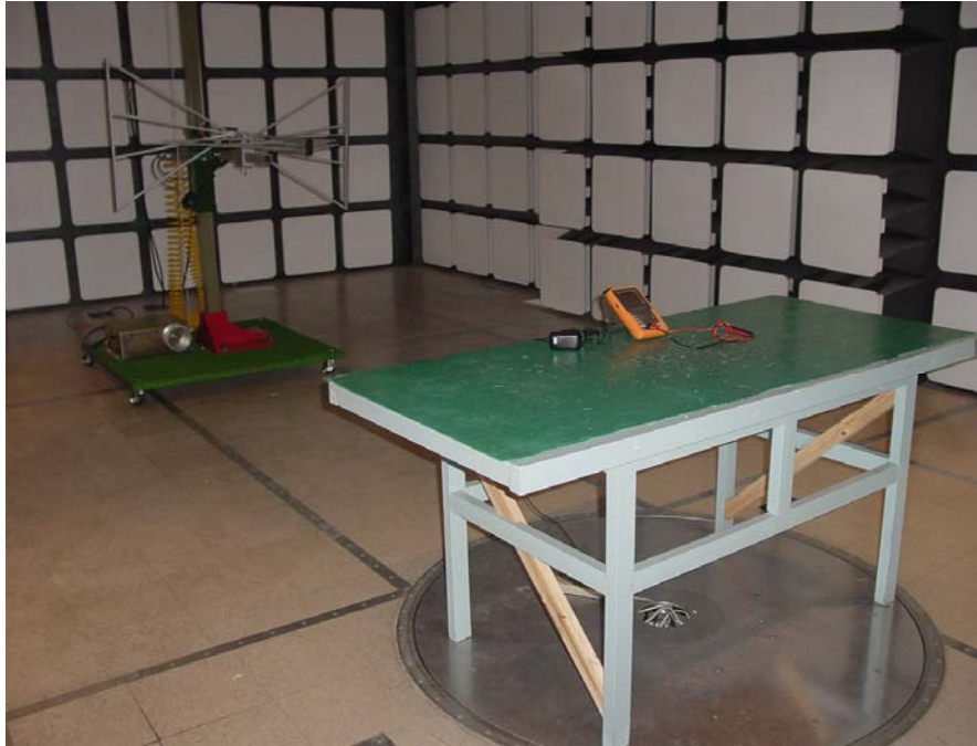
Radiated Emission Test Set-Up – Horizontal View
