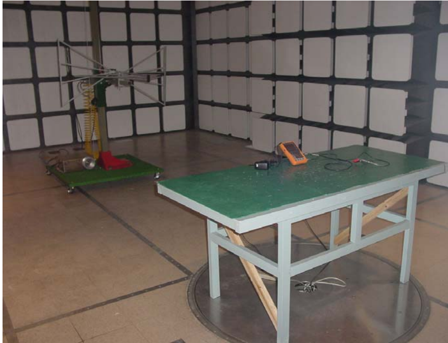
Radiated Emission Test Set-Up – Horizontal View
