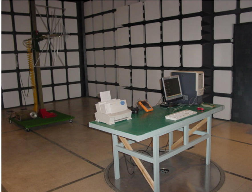
Radiated Emission Test Set-Up – Vertical View
