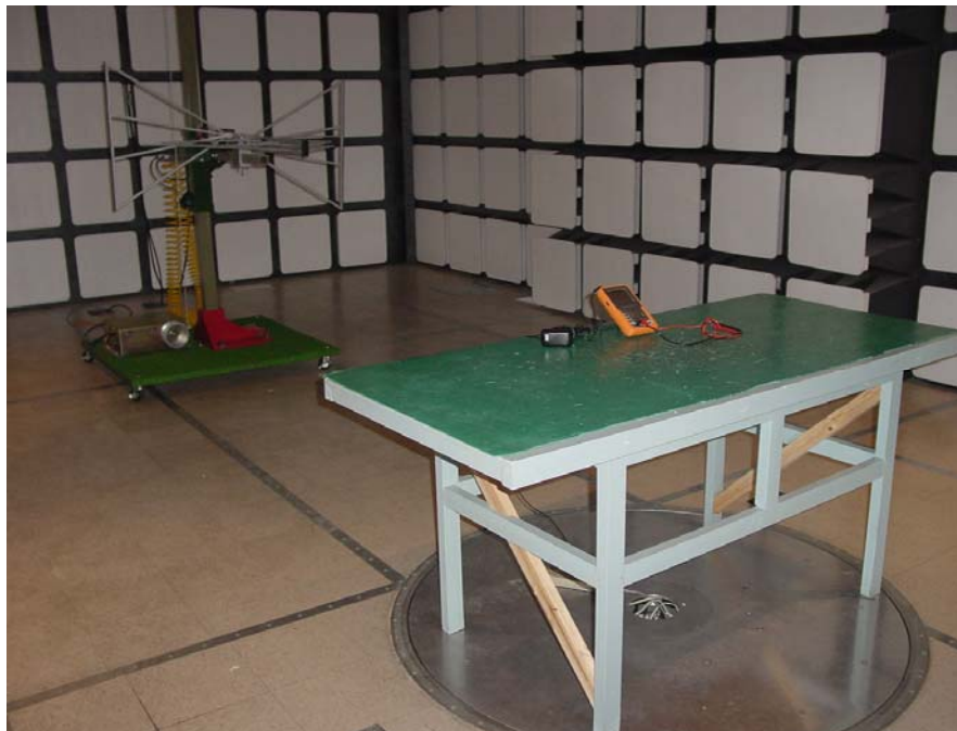
Radiated Emission Test Set-Up - Horizontal View
