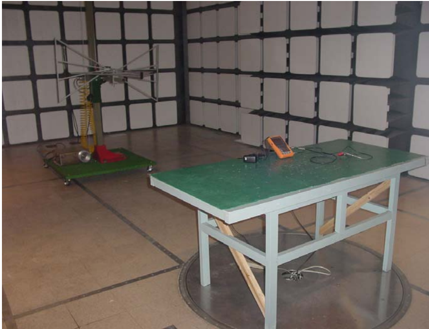
Radiated Emission Test Set-Up - Horizontal View
