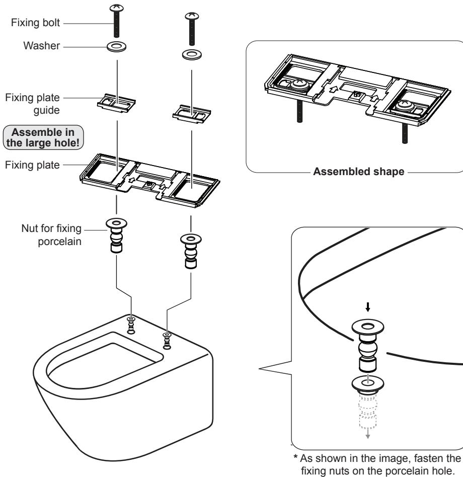
4. Insert the fixing plate set in the center of the rear of the main bidet unit to assemble.
