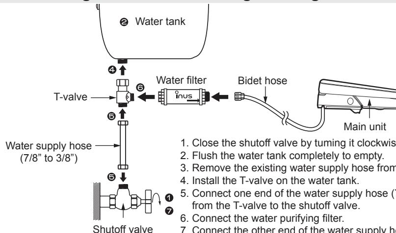
1. Close the shutoff valve by turning it clockwise.
