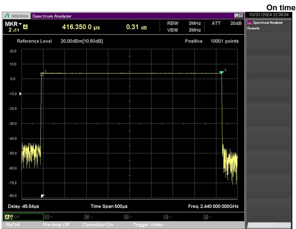
Note 1 : Duty Cycle Correction Factor(DCCF) =  $20 \log(\text{Duty cycle}) = -20.01 \text{ dB}$
