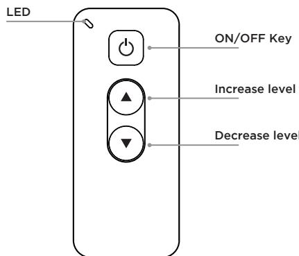
Fig. 1: Proflame Remote Control Plus
