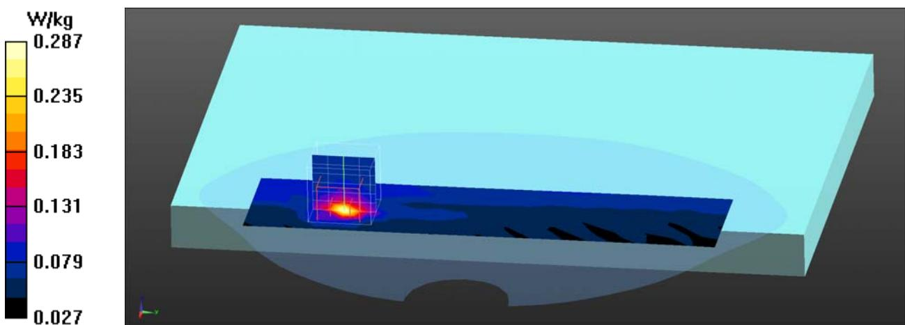
**802.11b EUT Back (Main Antenna) Z-Axis plot****Channel: 1**
