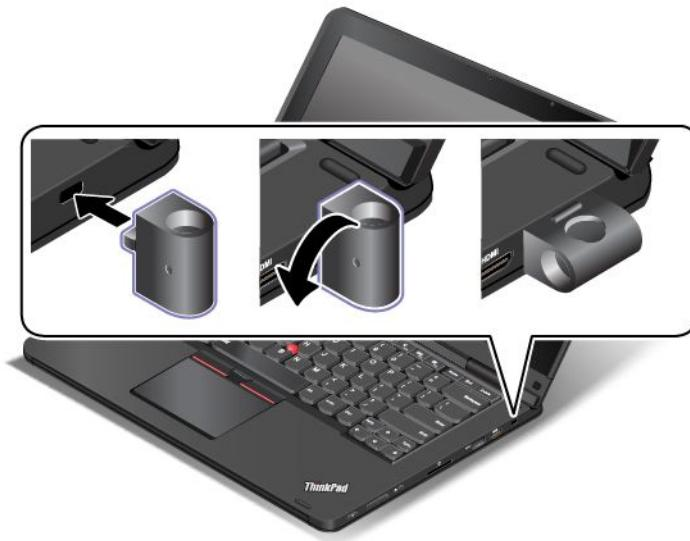
2. Insert the ThinkPad Active Capacitive Pen into any one of the three holes on the pen holder, as shown in the following illustrations:
