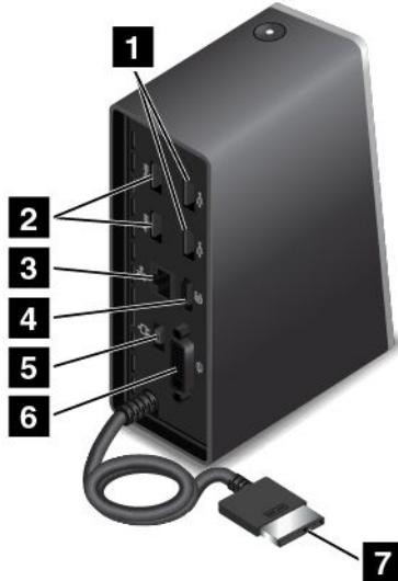
**1 USB 2.0 connectors:** Used to connect devices that are compatible with USB 2.0.
