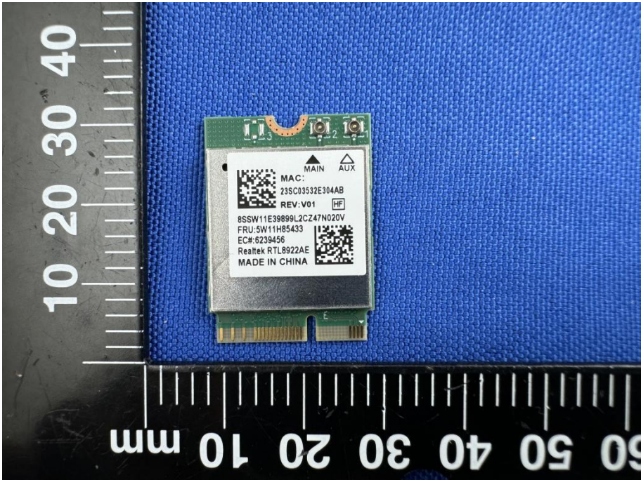
RF MODULE TOP VIEW-RTL8922AE(WITH SHIELDING)
