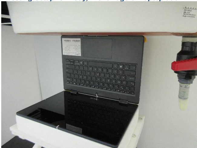
Testing Setup for Body, Top Side at 0 mm
