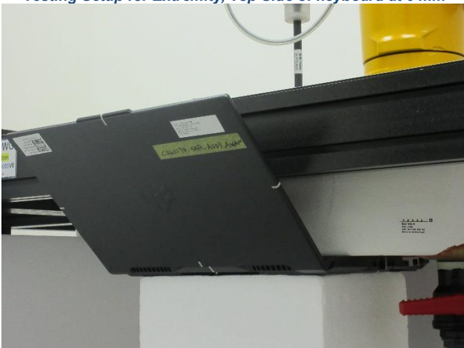
Testing Setup for Extremity, Top Side of keyboard at 0 mm
