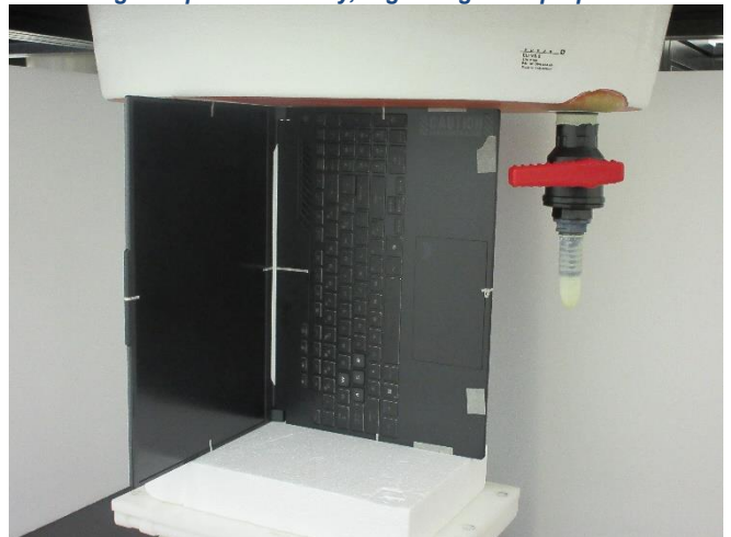
Testing Setup for Extremity, Right Edge of laptop at 0 mm
