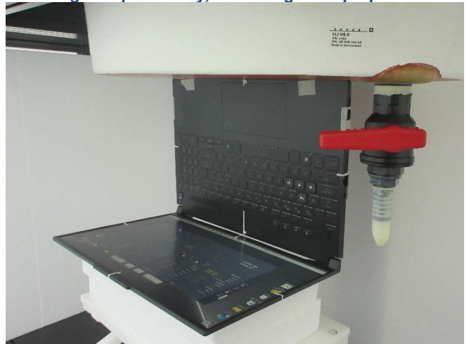
Testing Setup for Body, Front Edge of laptop at 0 mm
